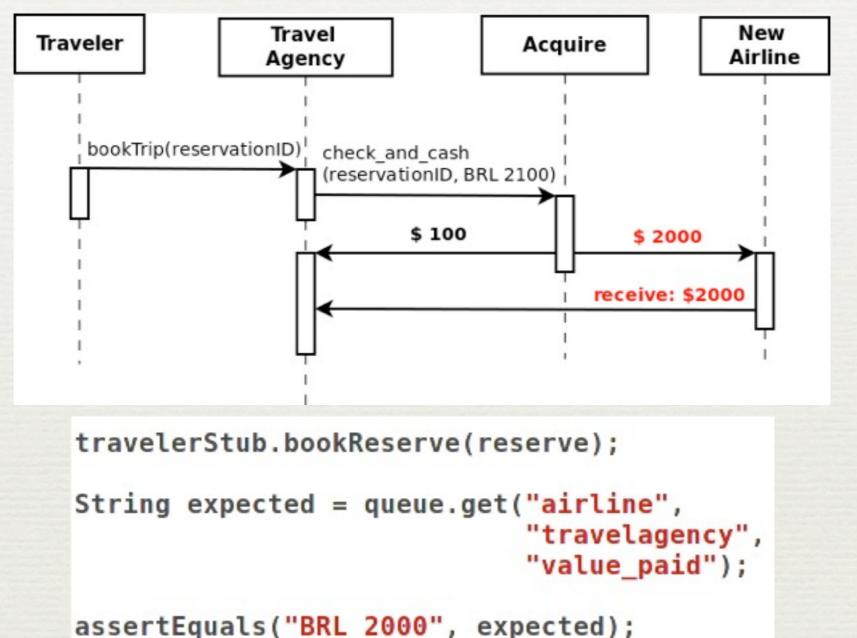
Example of a bug discovered by the integration testing technique
